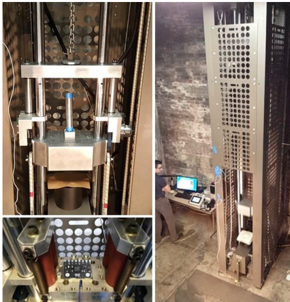
Figure 4: High-G Mechanical Shock Test Set-up. Shock system mounting table with test article (top left), Dual Mass Shock Amplifier (DMSA) with test article (bottom left) and mechanical shock system with a 16 ft tower (right).
